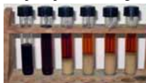
Samples of waste waters: untreated, treated with zeolite, treated with lime and treated with zeolite and lime together after centrifuging.
