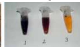
Views of the untreated waste water (1) waste water treated with zeolite 8 hours (2), waste water treated first with zeolite then lime 8 hours.
