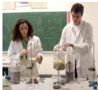
We first filtered these samples through glass wool then separated the olive oil from filtrate in separatory funnels.
